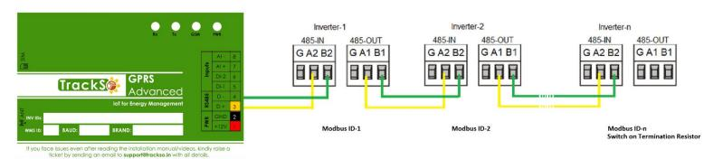
Note: At any one point of time only 1 Modbus Master-TrackSo Datalogger or Inverter Stick can be connected to Inverter for monitoring.
