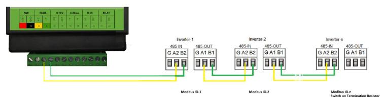
Note: At any one point of time only 1 Modbus Master- TrackSo Datalogger or Inverter Stick can be connected to Inverter for monitoring.
