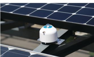
The MS-80S Class A pyranometer is designed for scientific research, industrial applications, photovoltaic system performance monitoring, and any application requiring the highest standard of accuracy possible.
