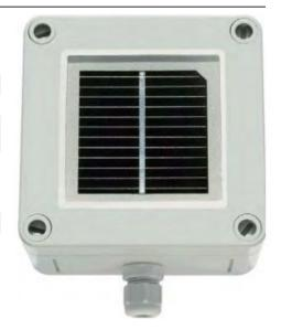
General Accuracy: NES Radiation Sensor Type SOZ-03 is better than 3% (from measuring value) in the range of 150-1200 W/m2 when the solar rays are perpendicular to the surface of the sensor and the spectrum corresponds to AM 1.5
