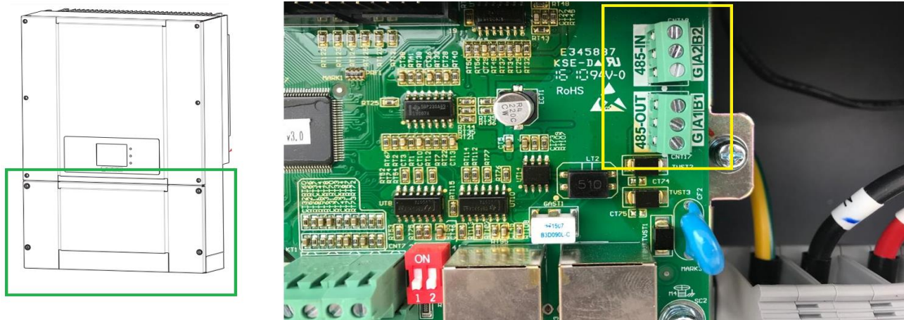
Figure S1: HITACHI String Inverter communication port & Connections
