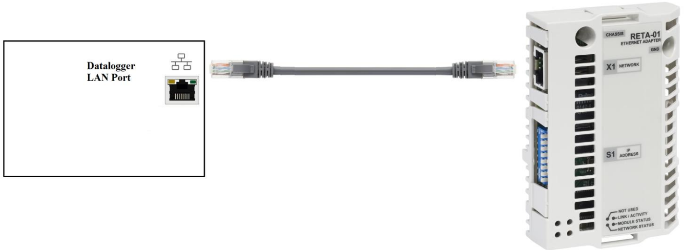
Figure A3- Connection of ABB Communication port with Ethernet based Datalogger
